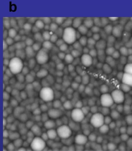
**Figure 1. AFM images of fluorocarbon coating deposited in from C<sub>2</sub>F<sub>4</sub> (flow rate 6 sccm; power 100W; pressure 200 mTorr) in MD conditions at different duty cycle values:**
