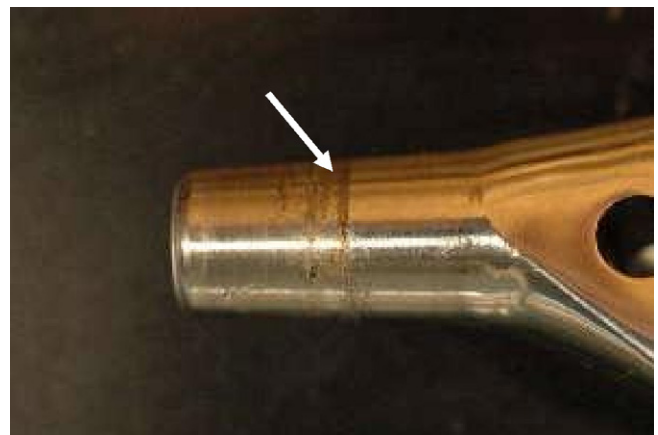
Fig. 5. Morse taper neck of a femoral Co–Cr stem corroded against a Co–Cr head in a non-cemented, modular early design. See the roughness of the Morse taper.
