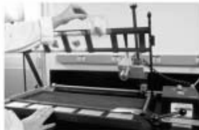
To prevent a grapevine sample for testing, sample material and buffer solution are sealed in plastic bags and loaded into a sack that holds them in place for grinding.
